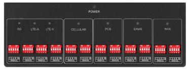
Switches should be OFF unless flashing red/yellow flashing lights occur for a channel or channels. Red/yellow flashing lights indicate the system has detected oscillation for the corresponding channel(s). They then turn off if adjustments are not made. When adjusting the booster, full power is not always the best option. Your goal is to obtain a usable signal in as many areas of the building as possible.
